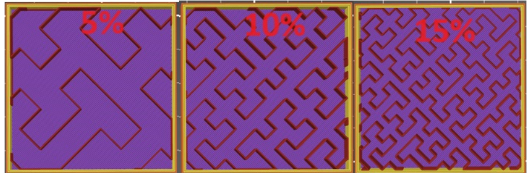
Figure 12. “Cross” geometry of pavement replica fillings (5%, 10%, and 15% of infill density).
