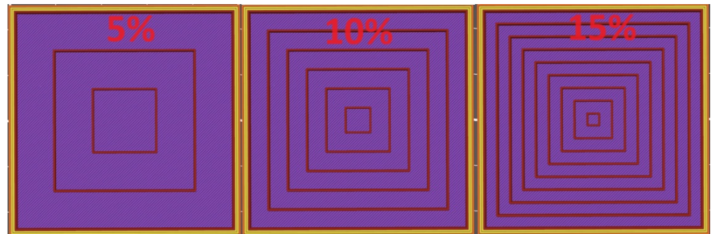
Figure 9. “Concentric” geometry of pavement replica fillings (5%, 10%, and 15% of infill density).
