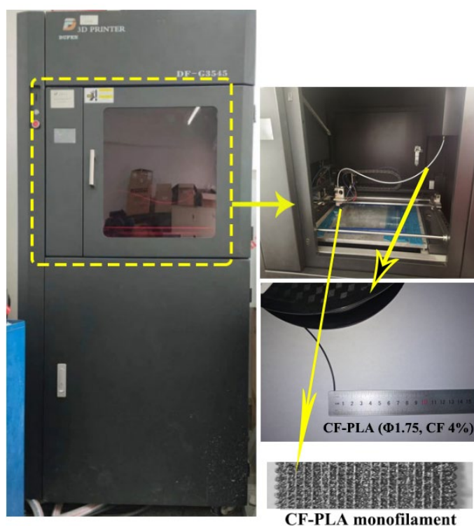
Figure 1. Three-dimensional printer for fabricating CF-PLA monofilaments.
