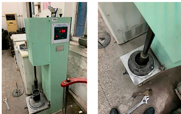
Figure 2. Impact test instrument (falling weight impact method).
