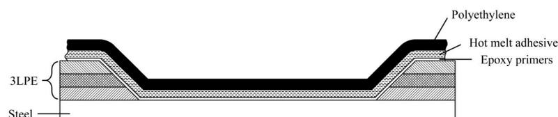
**Figure 9.** Schematic section of heat shrink tape bonded to the pipe.
