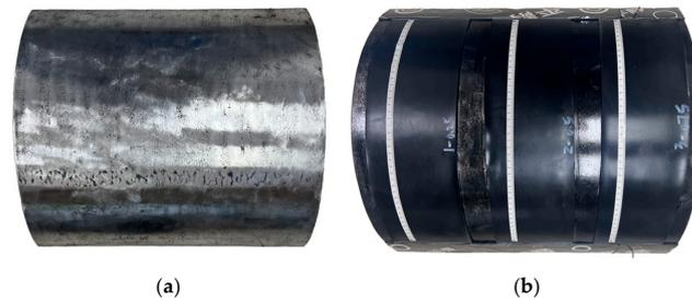
**Figure 10.** Test specimens: (a) Steel pipe after descaling; (b) Steel pipe after heat-shrinkable tape bonding.
