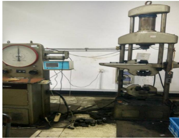
Figure 4. Hydraulic universal material splitting tester.
