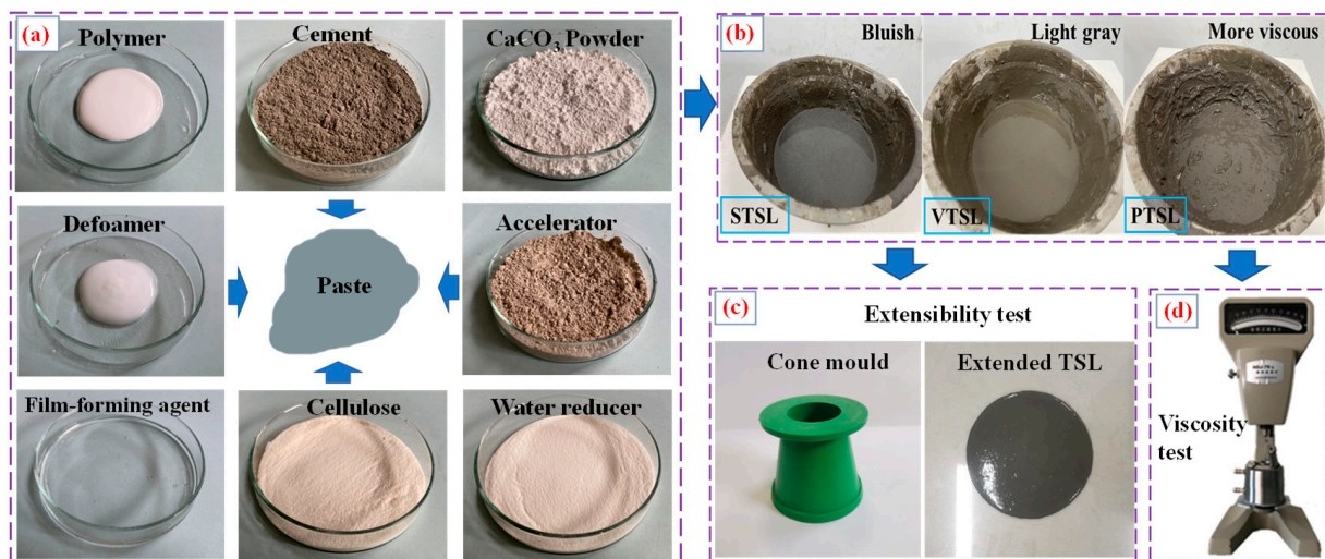
Figure 7. Extensibility test and viscosity test. (a): Raw materials for TSL preparation; (b): preparation of TSL slurry; (c): extensibility test; (d): viscosity test.
