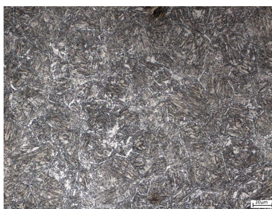
Figure 1. Metallographic structure of P110 casing steel.
