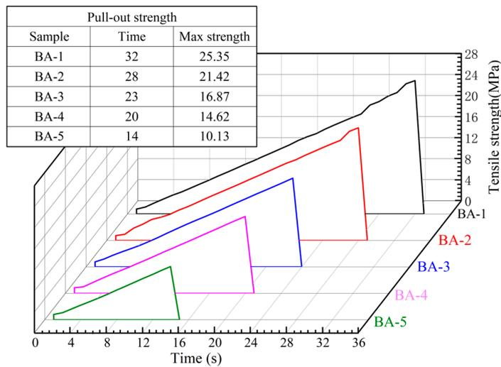
**Figure 6.** Quantitative results of different BAs obtained using the pull-out adhesion testing method.
