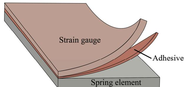
**Figure 1.** Schematic of an SG sensor.
