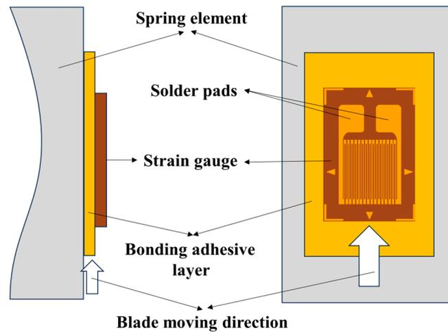
**Figure 2.** Illustration of blade moving direction and starting point location on the sensor.
