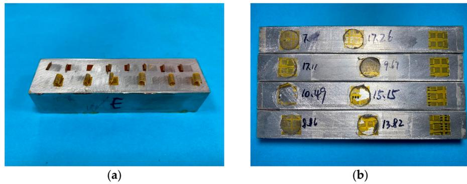
**Figure 5.** Shape of SG after scraping and drawing test: (a) Curl degree and curl height of SGs after scraper test; (b) SG after pull-out test.
