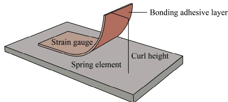
**Figure 3.** Schematic illustration of the curl height.
