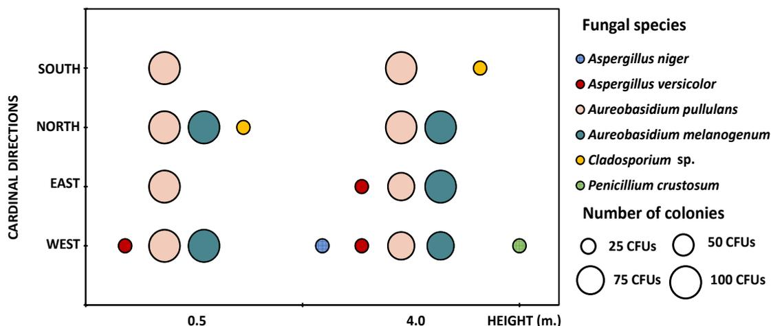
**Figure 3.** Culturable fungal colonies and fungal species identified on the Biofinish-coated facade after a 9-month exposure period at heights of 0.5 and 4 m from all four cardinal directions (north, south, east, west) of the building.
