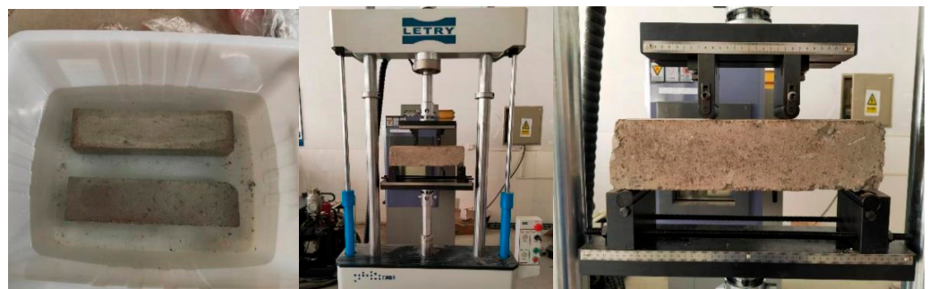
Figure 4. The four-point bending test apparatus.
