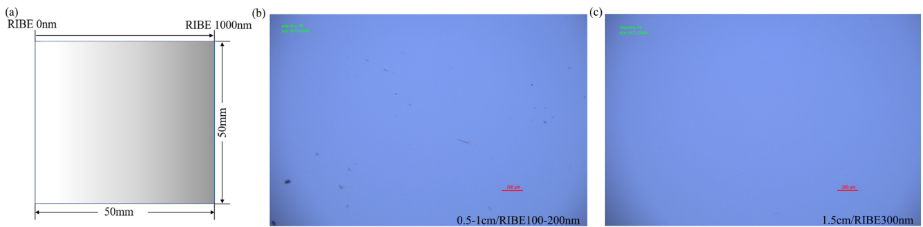
Figure 3. Ramp etching principle and shape. (a) A schematic diagram of the ramp etching process; (b) the surface profile of an optical element etched at 100–200 nm and 6–10 mm of the ramp element; and (c) the surface profile of an optical element etched at 300 nm at 15 mm of the ramp element.
