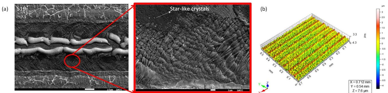
**Figure 11.** (a) SEM images of feather-like texture-covered sample S19. (b) 3D surface structure of S19.
