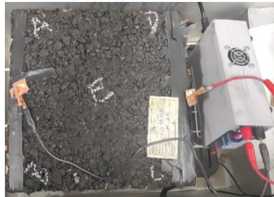
Figure 13. Temperature rise test of rutting slabs.
