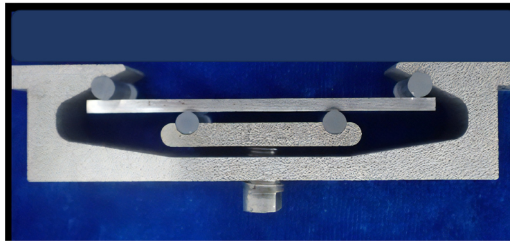
Figure 2. Four-point bending method with stress loading: physical image of the fixture.
