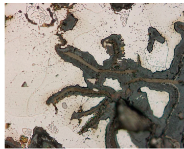
Figure 5. Microscopic image of selective corrosion on cast iron (magnification 500×) [3].
