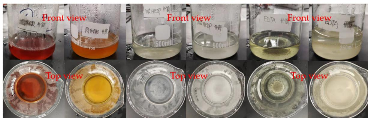
Figure 9. Corrosion results of retarded acid (from left to right: solid acid, HEDP, and EDTA).
