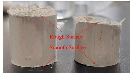
**Figure 15.** Core picture before acid solution.
