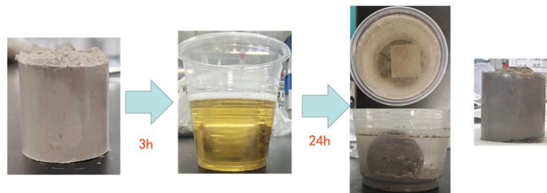
**Figure 16.** The overall acid corrosion effect diagram of the No. 1 core.
