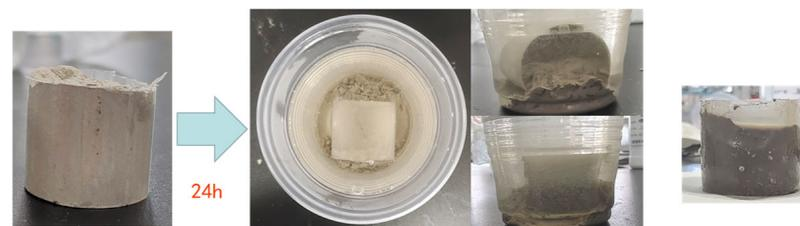
**Figure 17.** The overall acid corrosion effect diagram of the No. 2 core.
