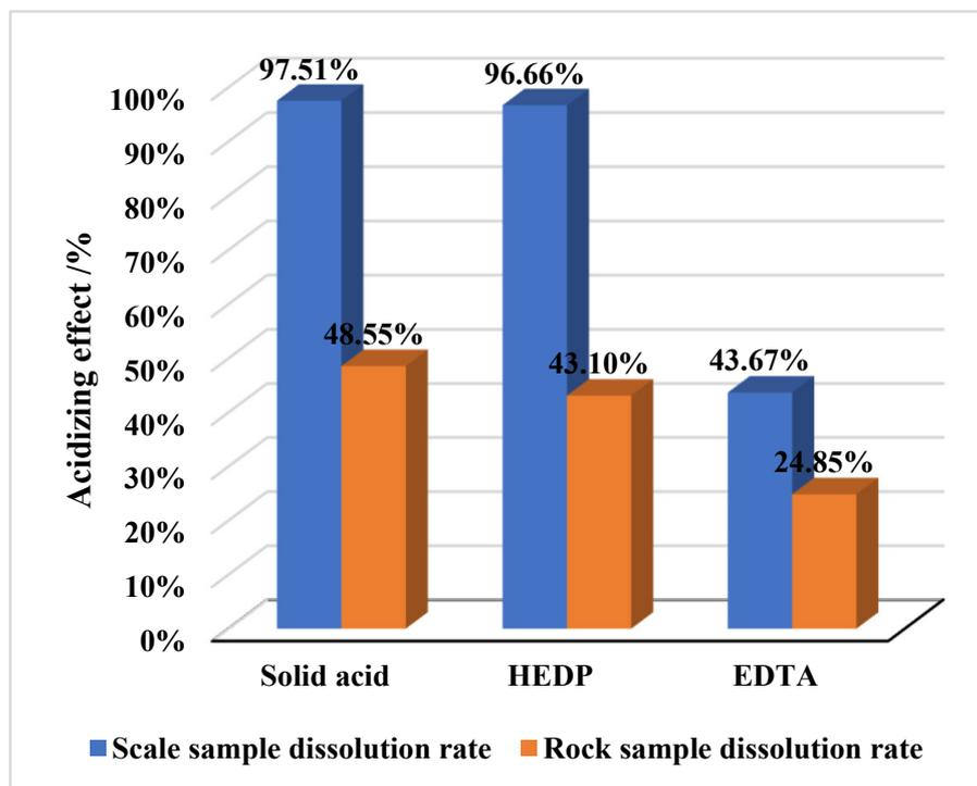
Figure 8. Corrosion results of retarded acid solution.
