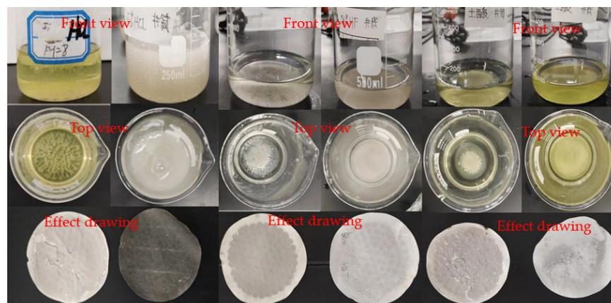
Figure 7. Results of acid dissolution (from left to right: hydrochloric acid, hydrofluoric acid, and mud acid).
