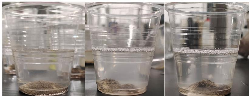
Figure 11. KCl solution immersion experiment (from left to right, 1% KCl, 2% KCl, and 4% KCl).
