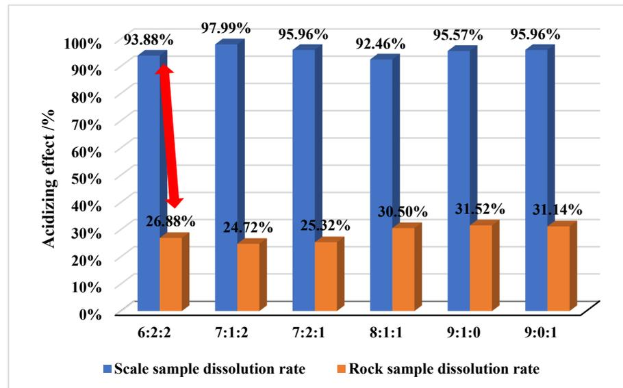
Figure 10. Corrosion results of complex acid solution.
