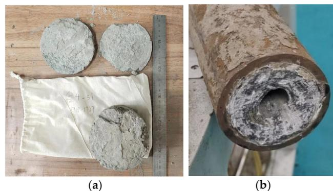
**Figure 3.** Reservoir rock and scale samples ((a): reservoir rock; (b): oil pipe scale).
