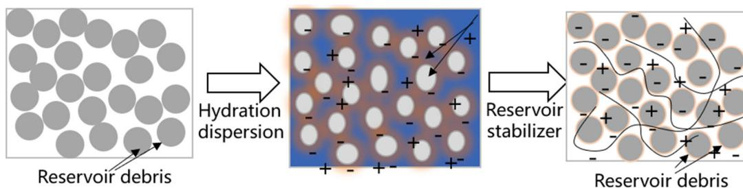
**Figure 5.** Schematic diagram of anti-dispersion principle of reservoir stabilizer.
