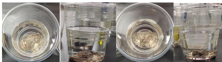
**Figure 13.** Surfactant immersion experiment (from left to right, nano-emulsion and Dodecyl pyridine chloride).
