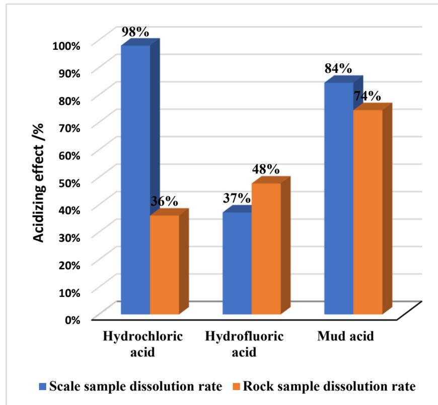
Figure 6. Corrosion results of conventional acid solution.
