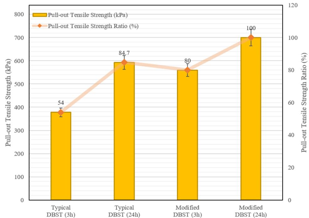
**Figure 7.** BBS test result comparison for typical and modified DBST after 3 h and 24 h of curing time.
