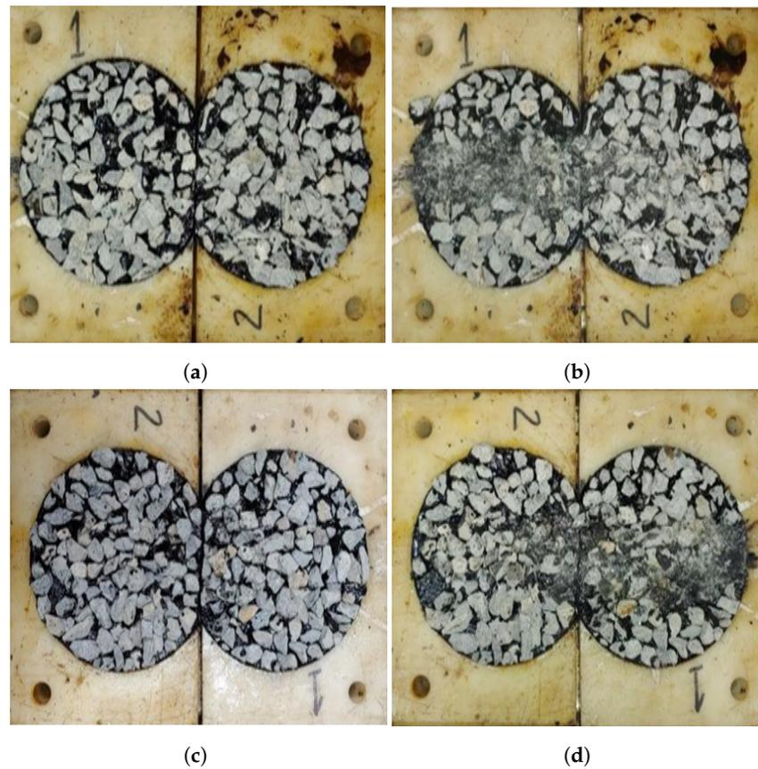
**Figure 11.** Visual comparison of specimens before and after 10 cycles of HWT loading. (a) Typical DBST before loading. (b) Typical DBST after loading. (c) Modified DBST before loading. (d) Polymer-modified DBST after loading.
