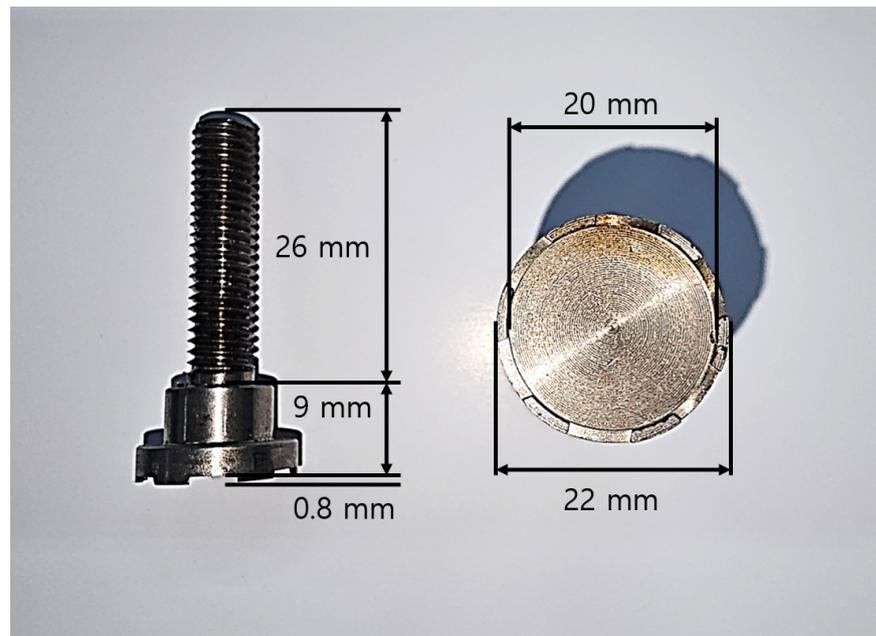
Figure 2. Pull-off stub geometry in mm.
