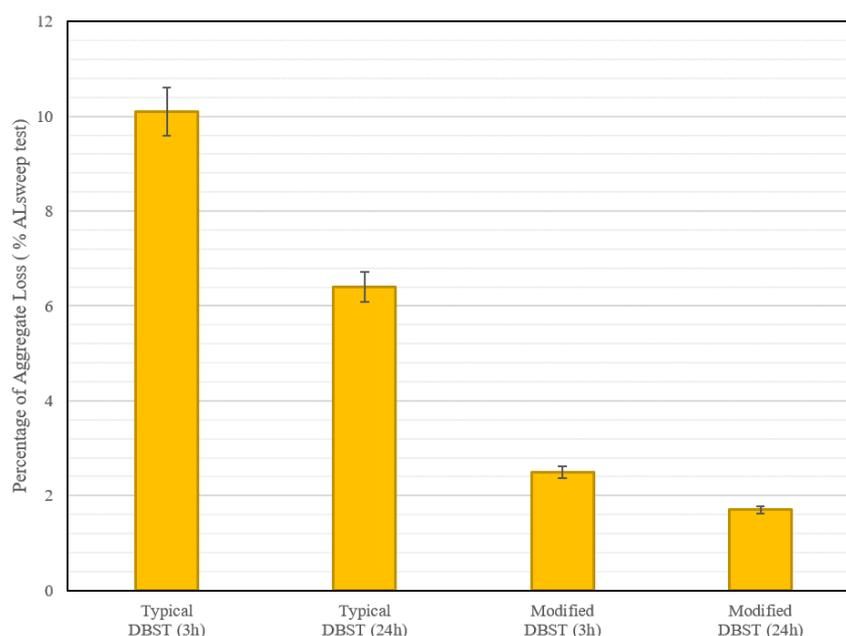
**Figure 10.** Sweep test result comparison for typical and modified DBST after 3 h and 24 h of curing time.
