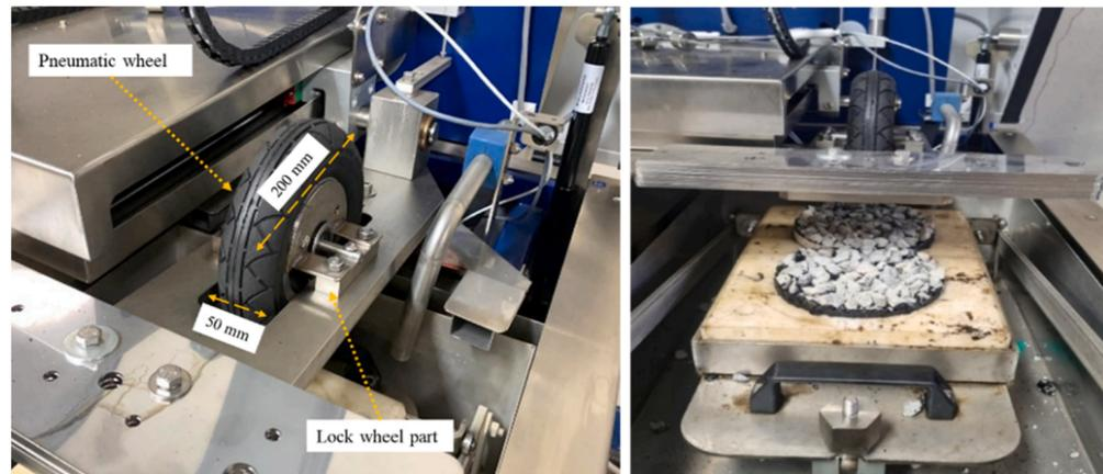
**Figure 5.** HWT test setup.
