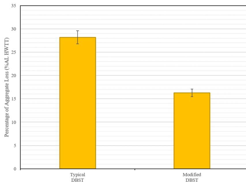
**Figure 12.** HWT test results for typical and modified DBST.
