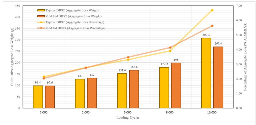
Figure 13. MMLS3 test results for typical and modified DBST.
