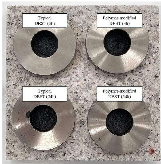
**Figure 8.** Failure modes of the specimens after the BBS test.
