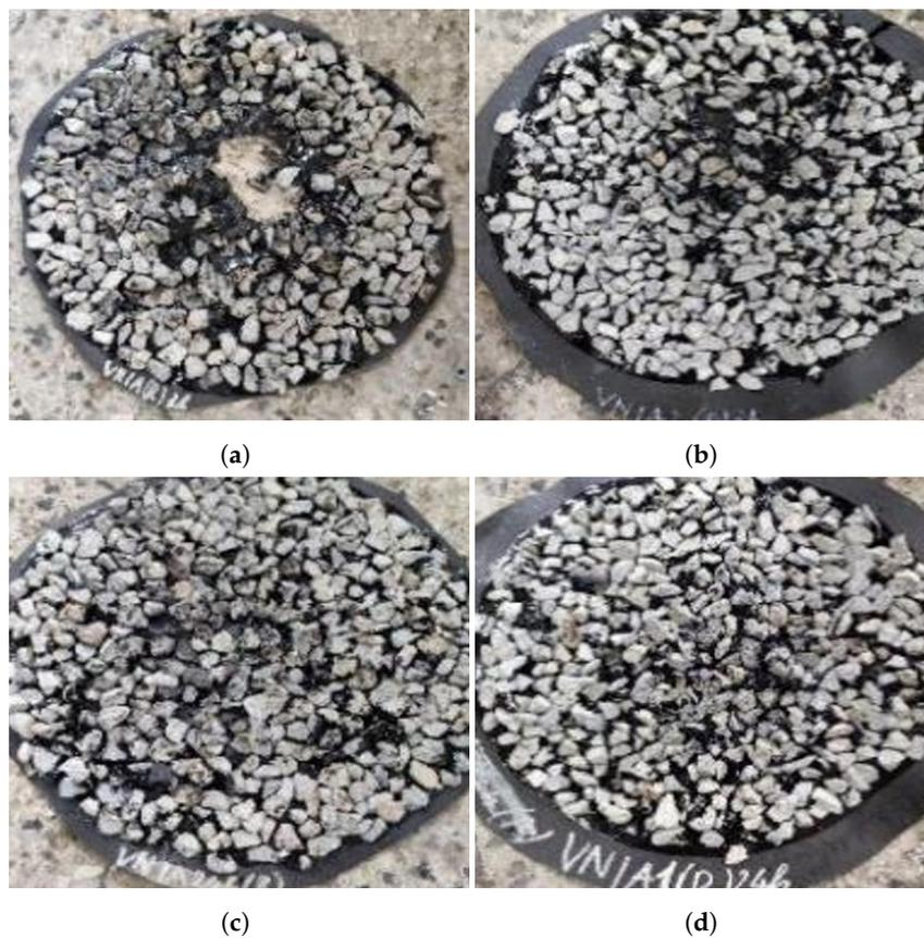
**Figure 9.** Test specimens after the sweep test. (a) Typical DBST (3 h). (b) Typical DBST (24 h). (c) Modified DBST (3 h). (d) Modified DBST (24 h).
