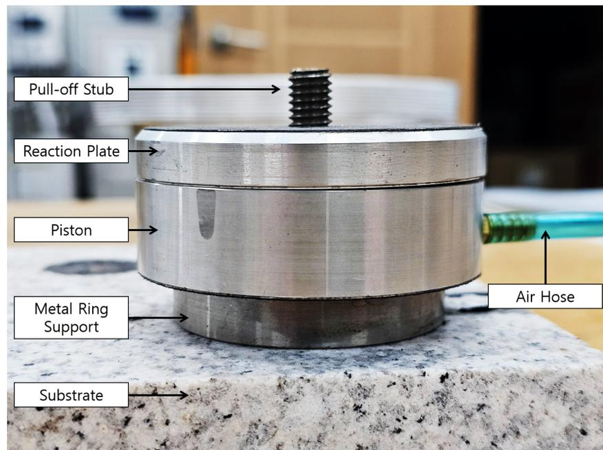
Figure 3. BBS test setup.
