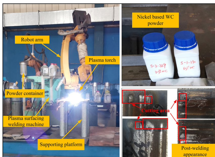
Figure 6. Experimental results of plasma surfacing welding.
