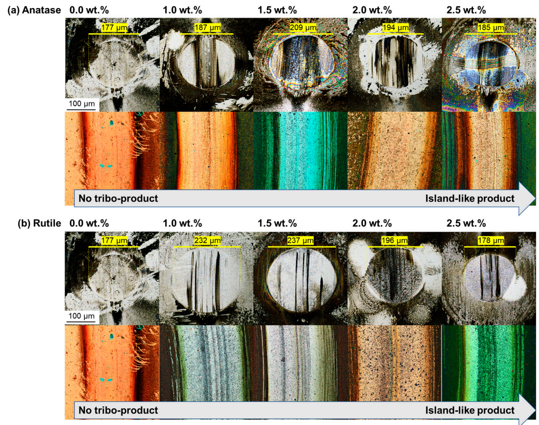
Figure 5. Optical images of wear track on ta-C disk and wear scar of steel ball after friction test under PAO4 mixed with MoDTC 700 ppm and TDONPs: (a) a-TDONPs and (b) r-TDONPs.
