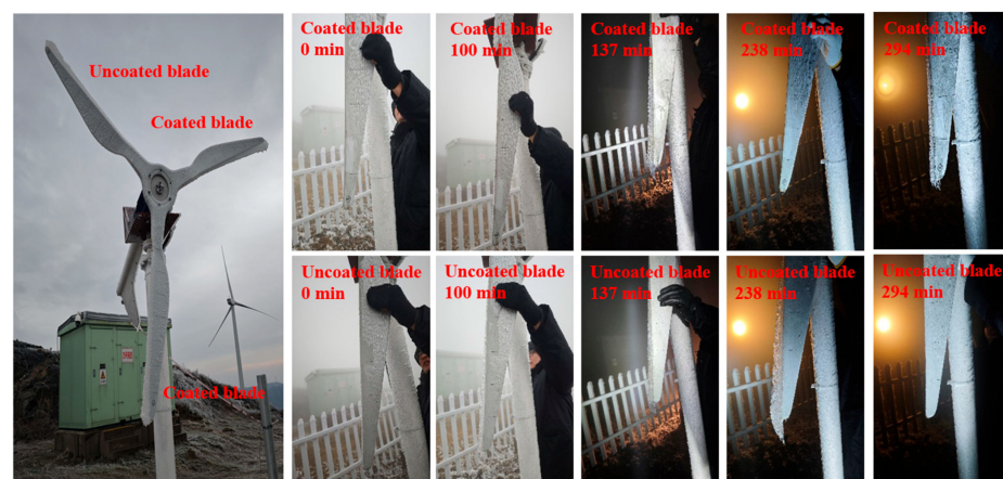
Figure 15. Ice accumulation and distribution on the coated and uncoated small wind turbine blades.
