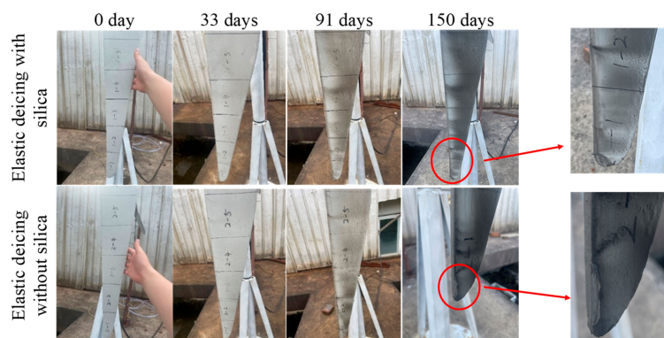
Figure 6. Outdoor aging behavior of elastic deicing coatings with and without silica.
