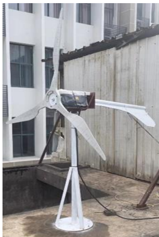
Figure S2. The wind fan used for the durability test of the elastic deicing coatings.
