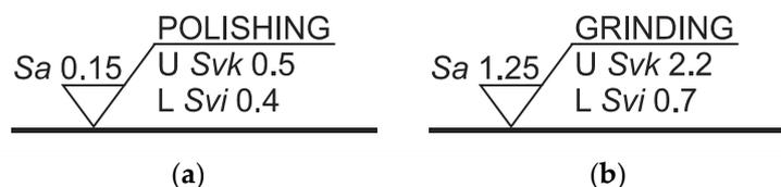
**Figure 14.** Description of the geometrical texture of the surface to provide similar strength of the adhesive joint when using: (a) T1 epoxy adhesive; (b) T2 cyanoacrylate adhesive.
