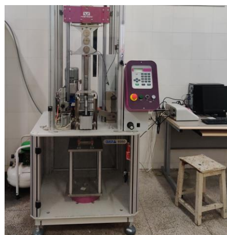
Figure 1. Instron CEAST 9350 and specimen for LVI test.
