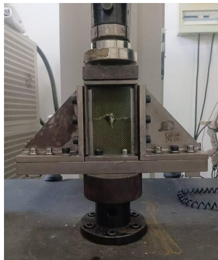
Figure 2. Test fixture and specimen of compression after impact.
