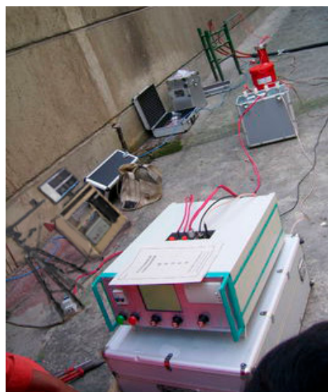
Figure 12. Experimental setup of the system used for detecting the thermal properties of the cables.
