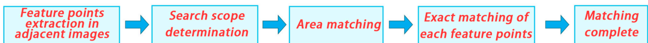
Figure 5. Proposed stitching method based on the combination of area matching and feature point matching.
