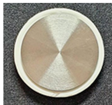
Figure 2. A blank sample put on the ceramic support ready for the thermal treatment.
