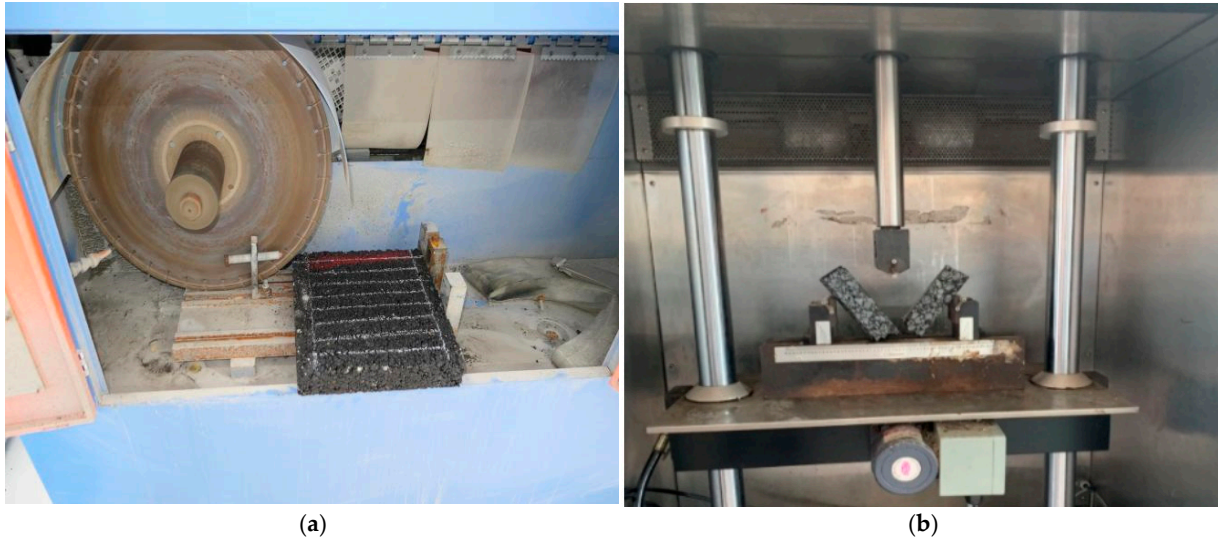
Figure 5. Low-temperature bending test. (a) cutting of beam specimens, (b) bending failure.
