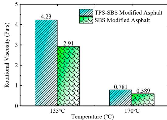
Figure 5. The rotational viscosity test values of asphalt.
