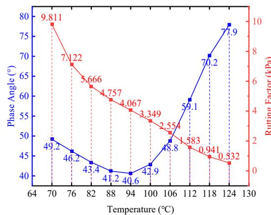
Figure 6. Temperature scanning test results of TPS-SBS modified asphalt.
