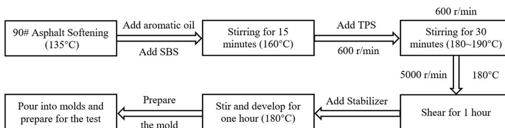
**Figure 1.** Preparation Workflow for TPS-SBS-Based High-Viscosity and High-Elasticity Modified Asphalt.
