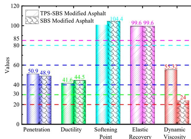
**Figure 4.** Basic Performance Test Results of Modified Asphalt (Note: The dashed lines in the figure represent the minimum technical limit values for the corresponding color performance. The range between the two blue dashed lines represents the technical specification range for the penetration value).
