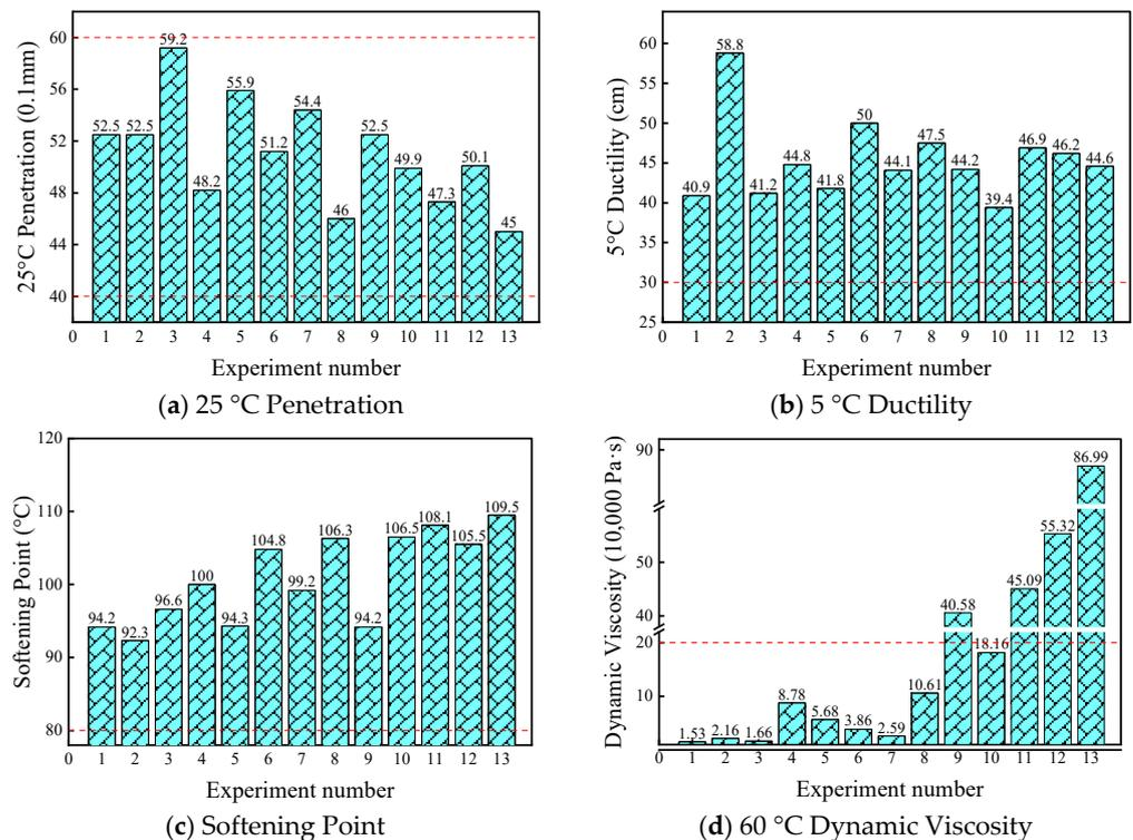
**Figure 2.** Performance Test Results of TPS-SBS High Viscosity and High Elasticity Modified Asphalt (Note: The test numbers in the figure correspond to those in Tables 6 and 8, representing samples under the mix ratios in Tables 6 and 8. The red dashed line in the figure represents the technical specification range limit or the minimum limit).
