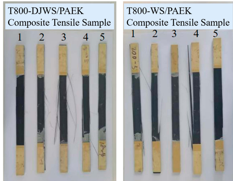
Figure 8. T800-DJWS/PAEK and T800-WS/PAEK composite samples that experienced tensile test failure.
