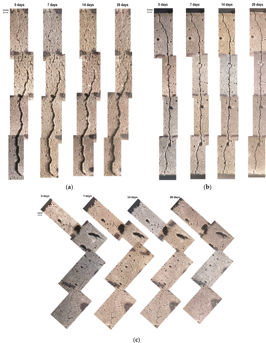
Figure 5. Crack healing progression on test bodies at 0 days, 7 days, 14 days, and 28 days of age with Soil B bacteria (a) IB3 Bacillus sp., (b) IB4 Citrobacter sp., and (c) IB5 Pseudomonas sp.
