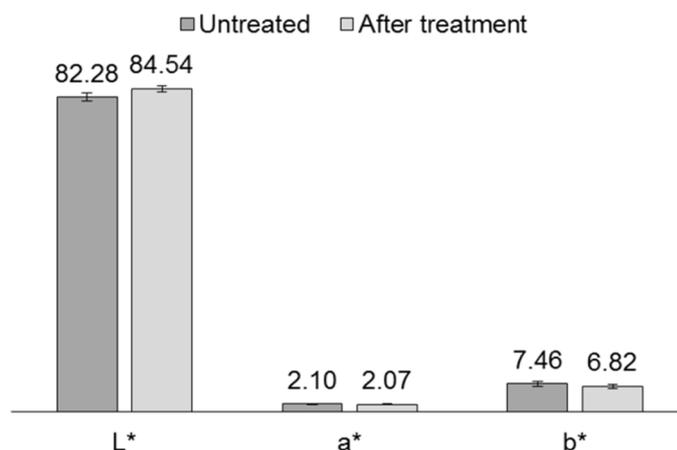
**Figure 3.** Average chromatic values according to CIELAB system before and after TiO<sub>2</sub> treatment.
