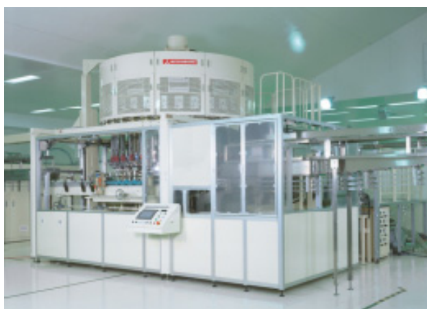
Figure 1. Example of high throughput rotary coating machine for PET bottles (photo provided by courtesy of Mitsubishi Heavy Industry Food and Package Co., Ltd., Nagoya, Japan).
