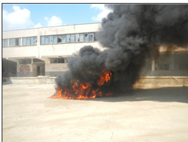
Figure 14. Fire of the 20 L gasoline on dense concrete pavement 15 s after ignition.
