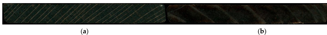
Figure 6. Penetration of PF resin into red oak (a) and radiata pine (b) panels treated with 30% PF-HALS resin. Note that the intensity of the blue-black colour caused by the reaction of ferric chloride with PF resin is less pronounced in the rays and earlywood of oak, and the latewood of pine, suggesting that penetration of the sample by PF resin was not uniform.
