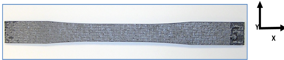
Figure 5. Optical photograph of an environmental barrier coating (EBC) coated melt infiltrated silicon carbide fiber reinforced silicon carbide matrix composite (MI SiC/SiC) composite dog bone specimen.
