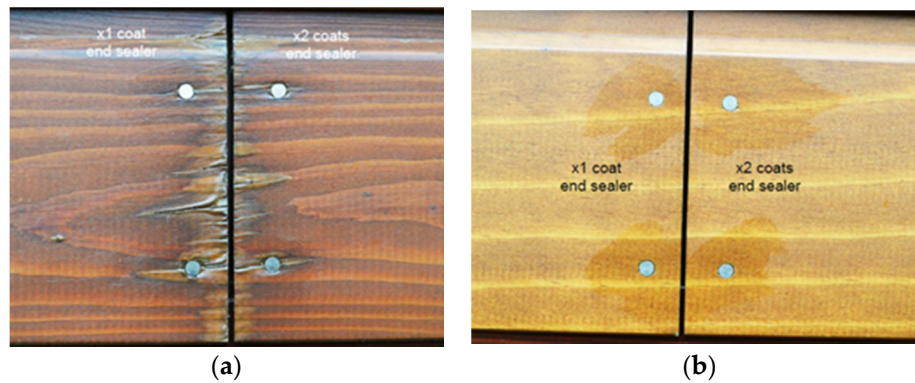
Figure 11. Control (larch, (a)) and acetylated (pine, (b)) samples after 7 years.
