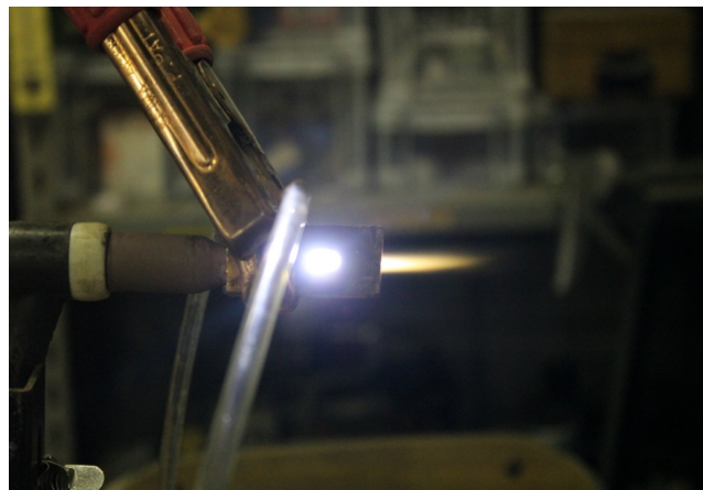
Figure 4. Plasma jet generated by our thermal spray equipment.
