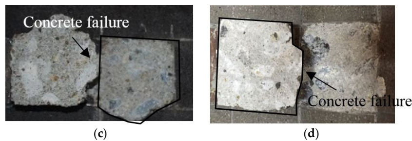
Figure 9. Failure mode depending on the surface treatment method: (a) sprayed, (b) abraded (c) sealed (A), and (d) sealed (B).
