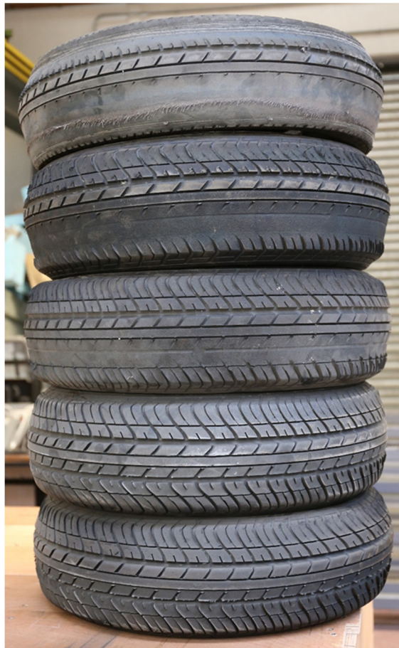
Figure 6. Stack of RTM tyres showing wear after 50,000 wheel-passes.
