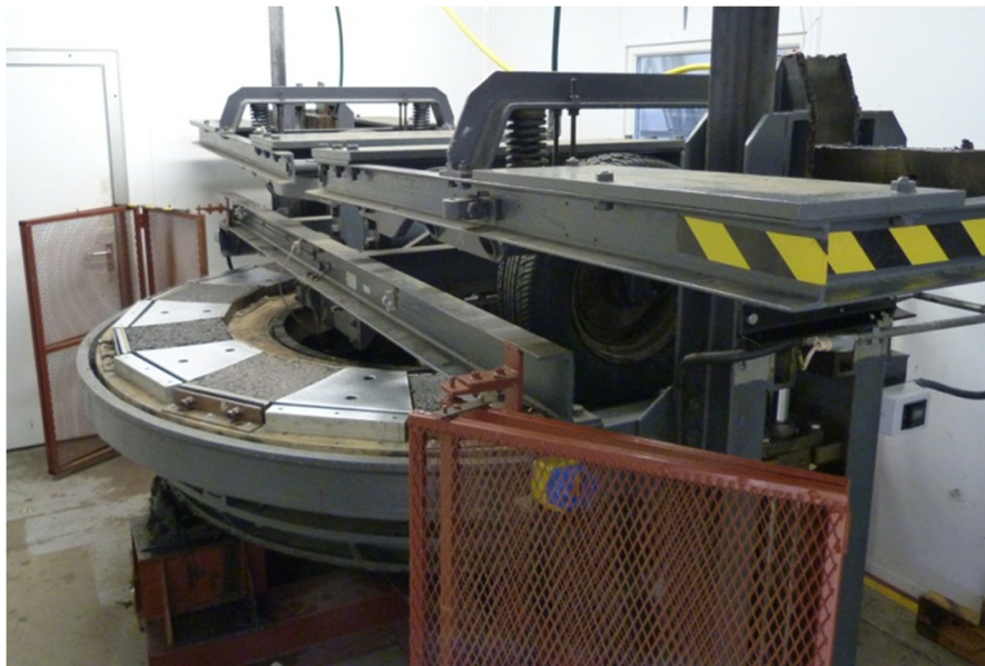
Figure 5. The Road Test Machine (RTM) used to test HFS for wear.
