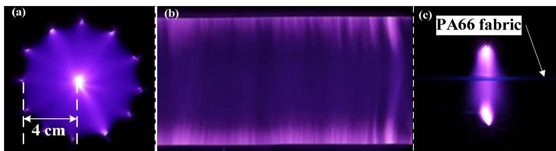
Figure 3. Images of the glow-like discharge: (a) The main view of the cylindrical electrode configuration in discharge; (b) The side view of the discharge with one pair of electrodes; (c) The PA66 fabric being treated.
