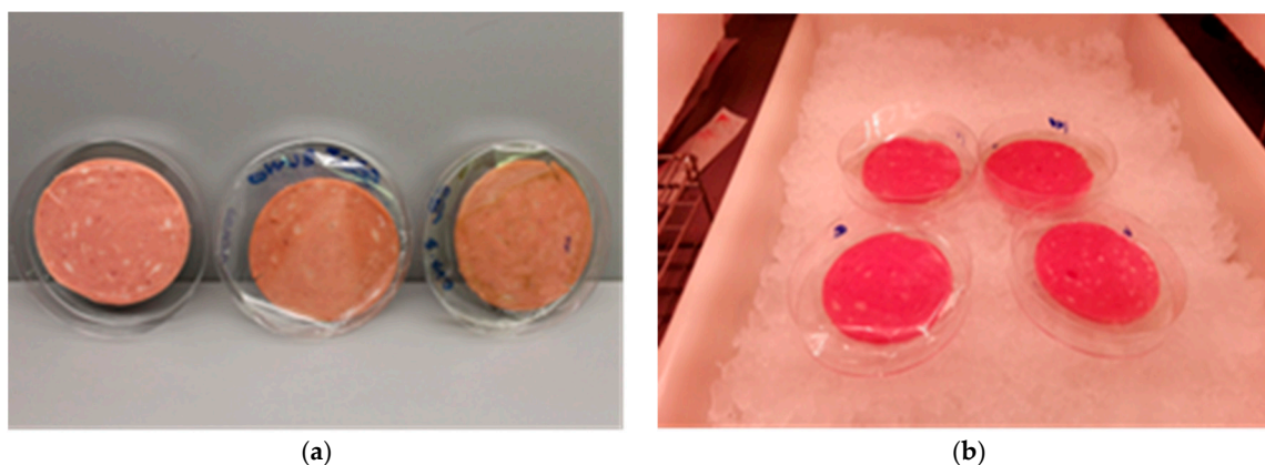
Figure 1. Example of test: (a) from left to right: bologna slice without coating, sample with a control gelatin (G) coating on poly(ethylene terephthalate) (PET), and sample of G-coated PET containing E-140 porphyrin; (b) image of an experiment of treatment during the photoactivation process.
