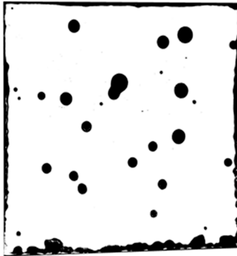
Figure 7. Binary image of Figure 8 to calculate the total corroded area.
