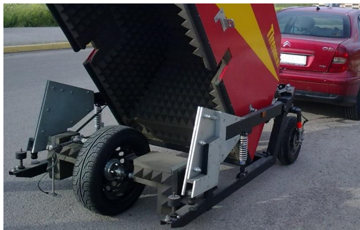
Figure 2. Reference tire inside the semi-anechoic chamber, and rear microphone.
