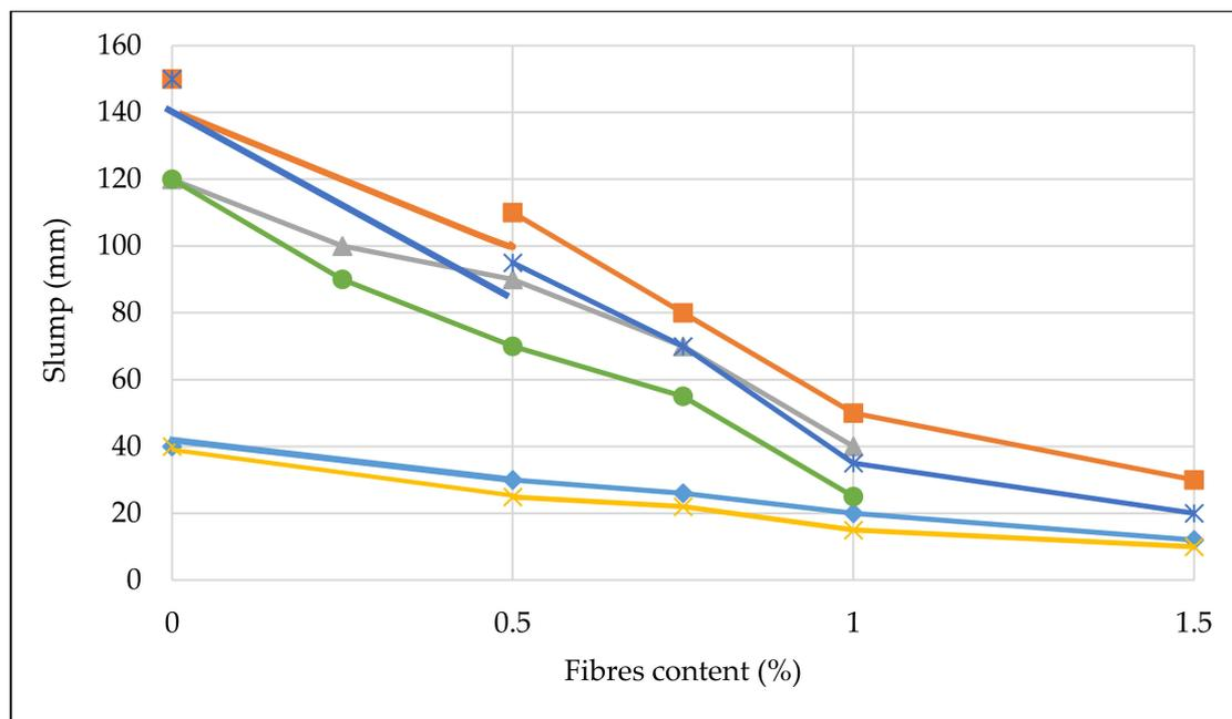
**Figure 8.** Influence of KF lengths and content on the workability of cement-based composites, data collected from the publications [35–37].
