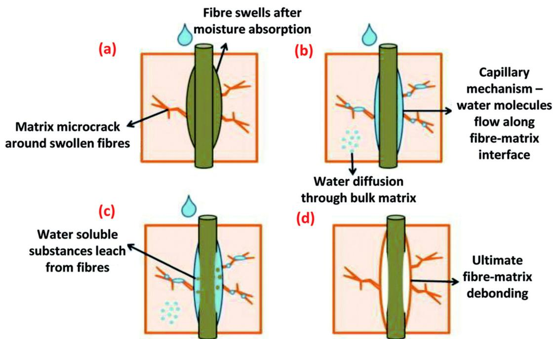
**Figure 6.** Effect of water on fibre–matrix interface. Reprinted from [33] with permission from Elsevier.
