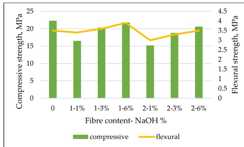
**Figure 10.** The effect of the sodium hydroxide (NaOH) solution and fibres content on the mechanical properties of KFRCC (data from [56]).
