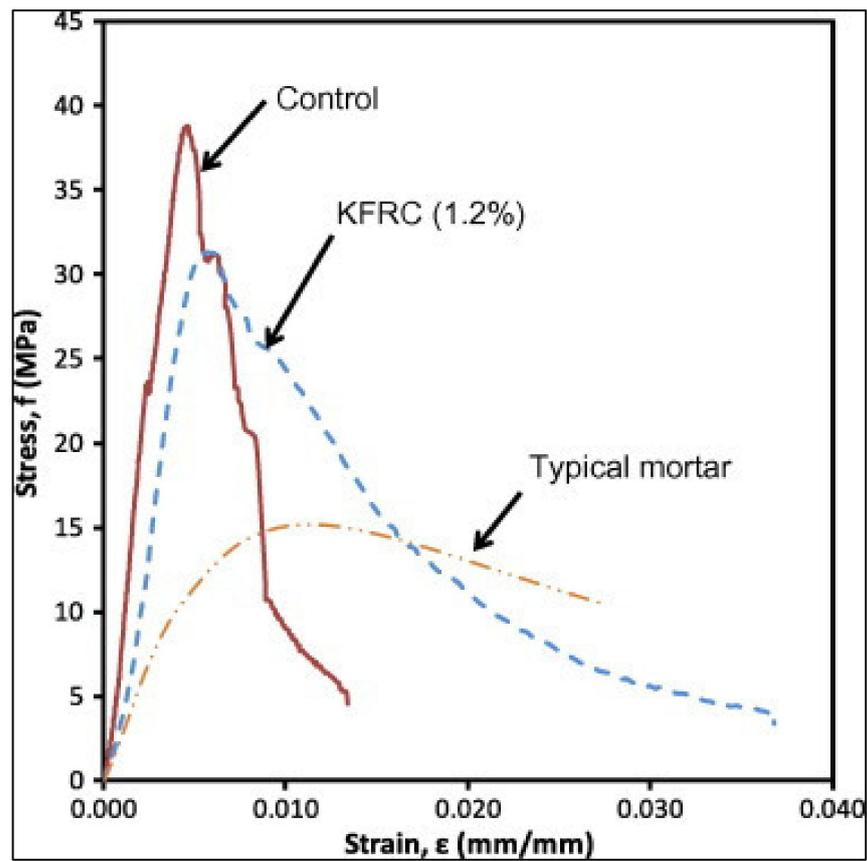
**Figure 11.** Stress-strain curve of the non-fibrous matrix (control) and KFRCC. Reprinted from [17] with permission from Elsevier.
