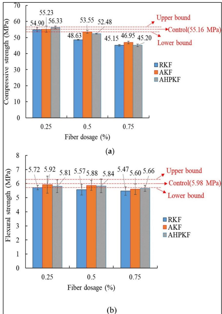
**Figure 9.** Impact of alkaline treatment method and fibre dosage on mechanical properties of KFRCC: (a) compressive strength and (b) flexural strength. Reprinted from [9] with permission from Elsevier.
