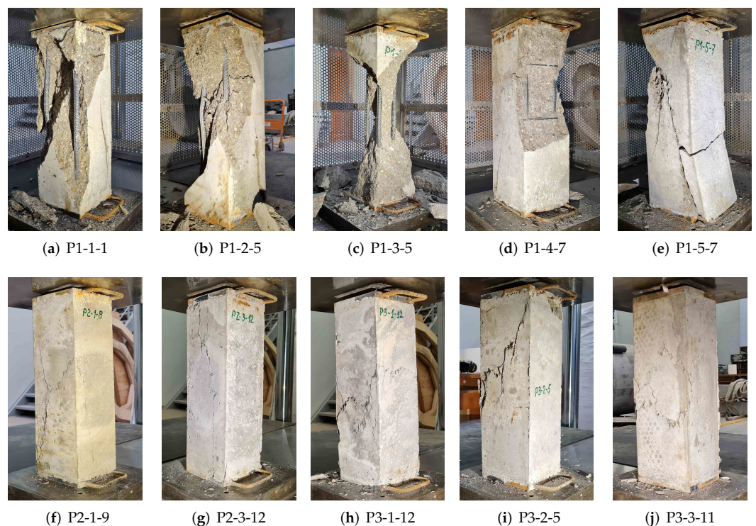
Figure 8. Typical failure modes of the tested samples: one specimen from each sample.
