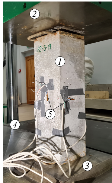
Figure 5. Test set-up: 1—test specimen; 2—loading head with ball-seat; 3—base plate; 4—machine frame; 5—strain gauges (for two specimens only).
