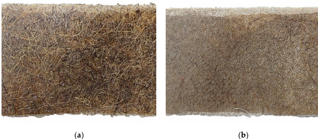
Figure 3. Composite samples: (a) hemp/PLA; (b) flax/PLA.
