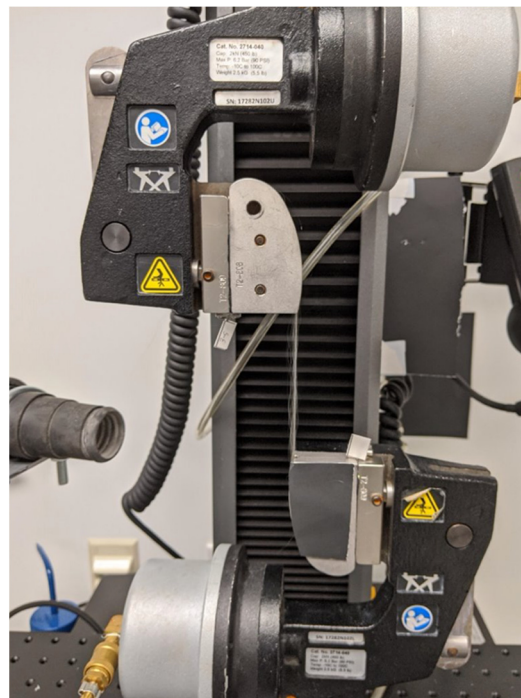
Figure 6. Yarn tensile testing experimental setup.
