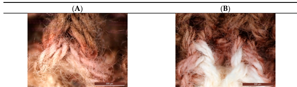
Figure 5. The comparison of images of the evidential material of sweater knitting damaged by the experimental action of diluted Domestos—(A); and original Domestos—(B).
