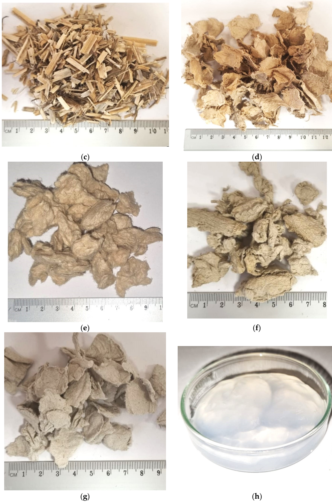
Figure 1. Materials used for paper composites: (a) Stems of hemp Cannabis sativa ; (b) Hemp stems after the decortication; (c) Hemp stems cut for pulping; (d) Hemp pulp; (e) Kraft pulp; (f) Waste pulp WF; (g) Waste pulp WFc; (h) Cellulose nanofibrils.
