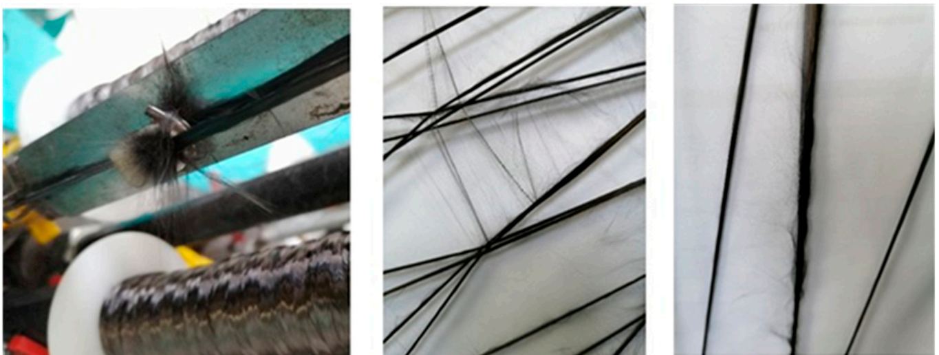
Figure 11. Different types of defects that can occur during braiding process.
