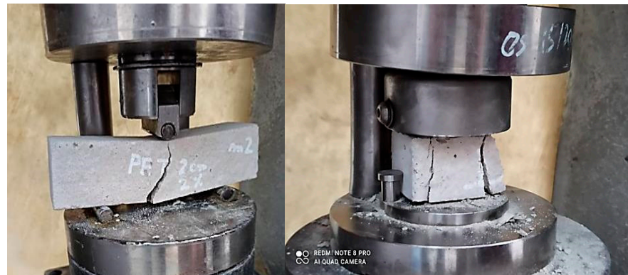
Figure 10. The mode of failure of sand concrete before exposure to high temperatures.
